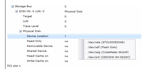
After initial selection the configuration description will only carry the actual device identifier (e.g. /dev/sdf ). You can always look up the long description by right clicking on the Device location line.
